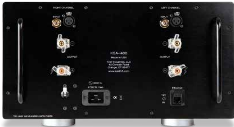
ABOVE: Large winged 4mm binding posts allow speaker cables and spades to be clamped firmly in place. Unswitched inputs are on RCAs and balanced XLRs. The 12V trigger facilitates system integration, but Ethernet port is for software updates only
